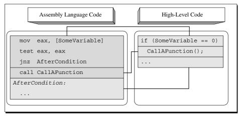
Figure A.1 High-level/low-level view of a single branch conditional sequence.
