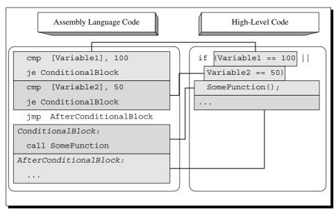
**Figure A.6** High-level/low-level view of a compound conditional statement with two conditions combined using the *OR* operator.
