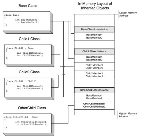
Figure C.5 Layout of inherited objects in memory.
