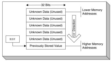
Figure 2.2 A view of the stack after the three values are popped out.
