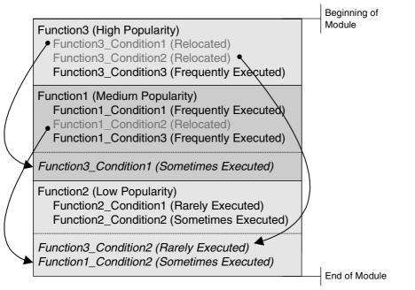
**Figure A.14** The effects of line-level working-set tuning on code placement in the same sample binary executable.
