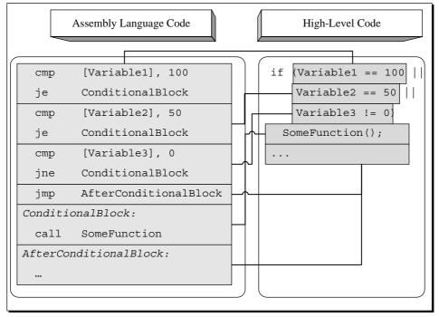
**Figure A.8** High-level/low-level view of a compound conditional statement with three conditions combined using the *OR* operator.
