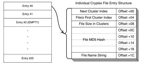
Figure 6.3 The format of a Cryptex file entry.
