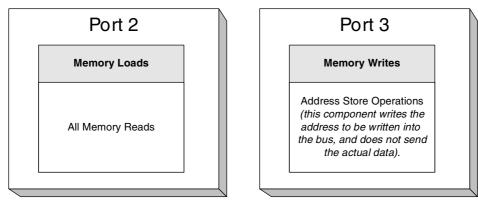
Figure 2.4 Issue ports and individual execution units in Intel NetBurst processors.
