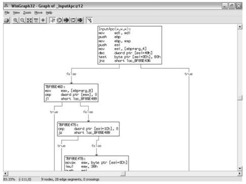
Figure 4.3 An IDA-generated function flowchart.
