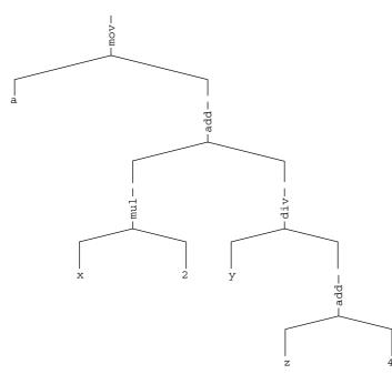
**Figure 13.1** An expression tree representing the above C high-level expression. The operators are expressed using their IA-32 instruction names to illustrate how such an expression is translated from a machine code representation to an expression tree.
