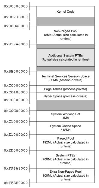
Figure 3.1 A typical layout of the Windows kernel memory address space.
