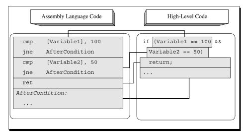
**Figure A.5** High-level/low-level view of a compound conditional statement with two conditions combined using the AND operator.
