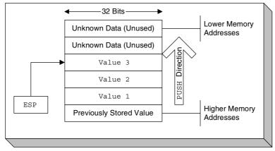
Figure 2.1 A view of the stack after three values are pushed in.
