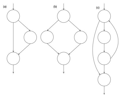
**Figure 13.2** Typical control flow graphs: (a) a simple if statement (b) an if-else statement (c) a while loop.
