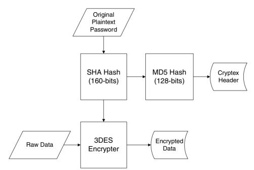
Figure 6.1 Cryptex's key-generation and password-verification process.
