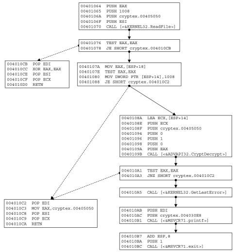
**Figure 13.3** An unstructured control flow graph representing branches in the original program. The dotted arrows represent conditional branch instructions while the plain ones represent fall-through cases—this is where execution proceeds when a branch isn't taken.
